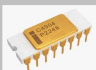
1971 – Microprocessor 2300 transistors – 10 μm
