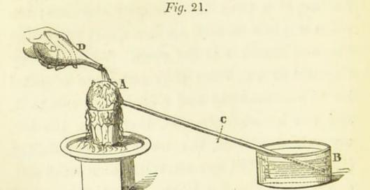
the tube from which dips into some coloured liquid in the vessel B. And I dare say you know that if I put my hand on the bulb A, and warm it, the coloured liquid which is now
