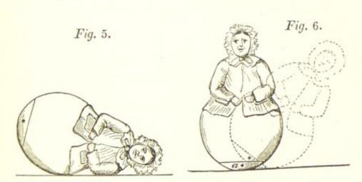
fectly sure, without looking inside the figure, that there is some arrangement by which the centre of gravity is at the lowest point when the image is standing upright; and we may be certain when I am tilting it over (see fig. 6) that I am lifting up the centre of gravity (a), and
