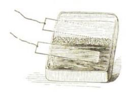
there is any difference in the two ends of the battery, and which it is that possess this peculiar action. You see it is the one on my right hand which has the power of destroying the blue, for the portion on that side is thoroughly bleached, while nothing has apparently occurred on the other side. I say apparently, for you must not imagine, that because you cannot perceive any action none has taken place.
