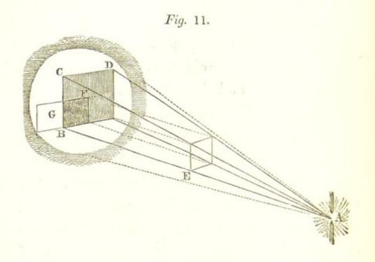
other one in size, and place it midway between the lamp and the screen; now look at the size of the shadow B D, it is four times the original size. Here, then, comes the "inverse square of the distance." This distance, A E, is one, and that distance, A B, is two; but that size E being one, this size B D of shadow is four instead of
