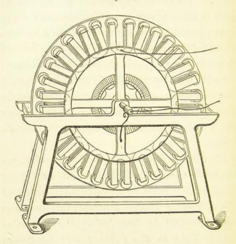
is the magneto-electric light, and an instrument has been constructed as there shown (fig. 59) which represents a number of magnets placed radially upon a wheel—three wheels of magnets
