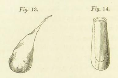
Here is another form of the same kind of experiment. I have here some more glass which has not been annealed [showing some thick glass vessels (11) (fig. 14)], and if I take one of these glass vessels and drop a piece of pounded glass into it (or I will take some of these small pieces of rock crystal—they have the advantage of being harder than glass) and
