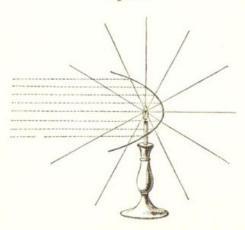
to be the rays of a candle or any other source of light emanating from the centre of a sphere in all directions round to infinite distances. After this simple kind of light had been used for some time, it being found to be liable to be obscured by fogs, or distance, or other circumstance, there arose the attempt to make larger
