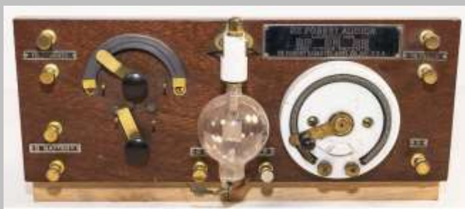
Fig. 5 – Detetor de rádio baseado no Audion / Radio detector based on Audion.
