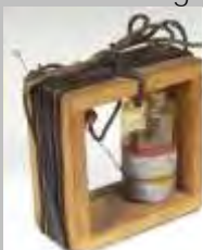
1899 – Marconi - ressonante circuito do 1º emissor / Marconi resonant circuit of 1st emitter.
