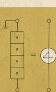
Schematic diagram of the four-layer transistor diode construction. Produced from single-crystal silicon, the four layers in the silicon unit are obtained by controlled diffusion of suitable impurities. Thickness is approximately 0.002 in.
