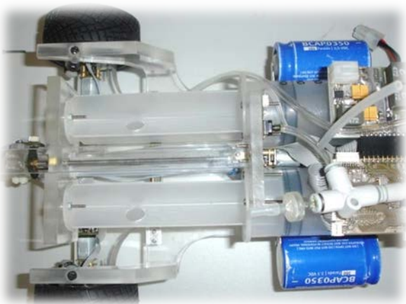
Fig. 11. Designed compressor with two pistons and a lead crew.
