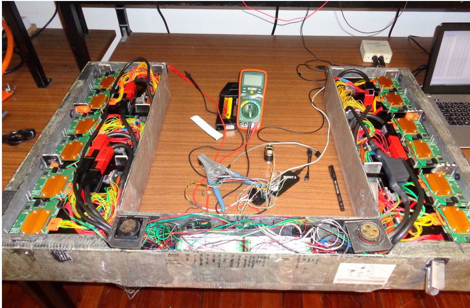
(a) Fully assembled battery without lid. Connector on the left of the middle section is low voltage only. Connector to the right is for high voltage and current.
