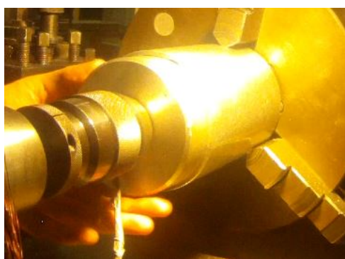
(c) Insertion of the rotor in the stator.
