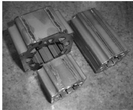
Figure 2.11: Stator welding as a stacking method [4].
