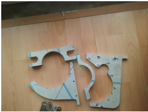
(a) Support pieces after waterjet cutting.
