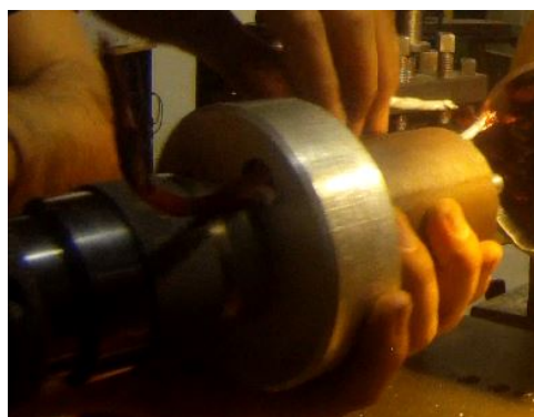
(b) Fixation of the shaft+bearing+front endplate in the tailstock.
